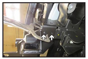
15. Using a 1/2" drill bit, drill out the bottom two (2) holes in the frame using the baseplate as a template. Insert two (2) 1/2" bolts with lock washers and whiz nuts. Do this on both sides of the vehicle.
