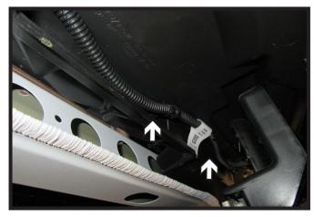
11. Remove the five (5) push pins from the bottom of the plastic shroud above the bumper. Unclip wire loom from the bottom of the shroud. Remove shroud and set aside to be reinstalled later.
