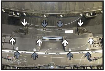
Using a 7MM socket, remove the six (6) bolts (white) from the cover on the back side of the fascia. Then remove the six (6) clips (gray). Remove cover from back of fascia, it will not be reinstalled.
