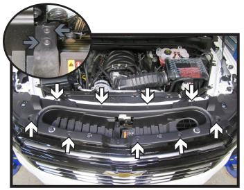
Remove the nine (9) push pins (white) from the fascia cover. Then using a T15 Torx, remove the two (2) screws from the hood latch handle (inset gray). Set aside the facia cover and hood latch handle to be re-installed later.
